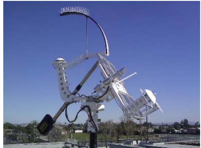
Two-axis test trackers for individual PV and concentrator module testing.
