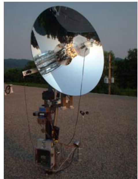
Fiberoptic concentrator daylighting – focuses light down fiber and delivers to internal rooms of a building.
