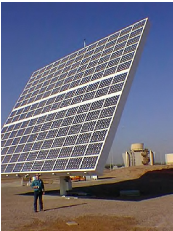
The Prospector™ – two-axis solar/weather station for monitoring and logging weather and solar influx and power output data.
