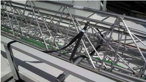
Remove the strap holding down the tower sections to the trailer bed. Keep it handy.
