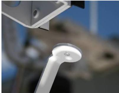
4. Use the joystick to move the Prospector until the dot of sunlight becomes a halo\*\*, perfectly centered on the hole in the back of the reflective pointer.
