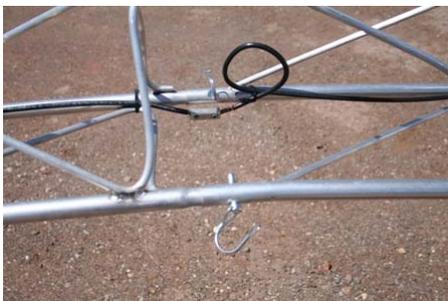
Insert the three locking pins then use the black strap to lash the two assembled pieces to the front of the trailer... the newer models have a convenient spare tire right there to accommodate... others have a rubber pad...
