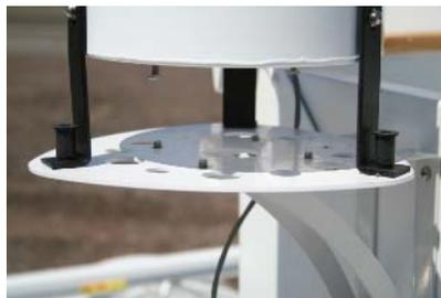
Remove the dust cap from the small receptacle beneath the mounting plate and attach the rain bucket signal cable.
