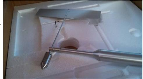
Each mast is labeled... the wind speed mast gets the anemometer cups and the wind direction gets the vane. The larger of the two hex wrenches is for the set screws in the mounting sleeves on the tower crossbar...
