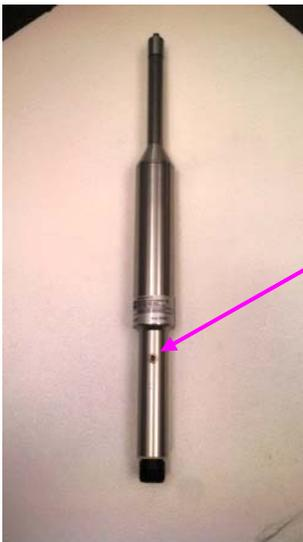
The wind direction sensor has a screw plug near the bottom that indicates where south is according to the reading from the instrument... in the northern hemisphere it will be oriented straight down or up in the southern hemisphere.
