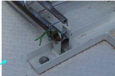
Undo the twisted wire at the hinge base of the tower and remove the pin holding in the grounding rod... this pin will go in the third mount to hold the tower upright.
