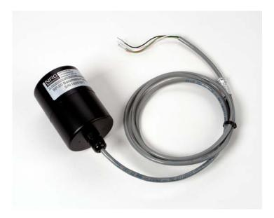
The NRG #BP20 barometric pressure sensor is a micromachined absolute pressure sensor which provides a high level voltage output signal that is proportional to absolute pressure. It includes built-in temperature compensation, linearization, and an output amplifier.
